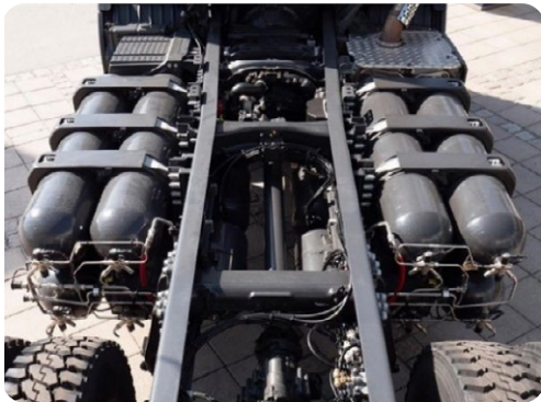
Fig. 1 CNG-tank in frame op chassis
